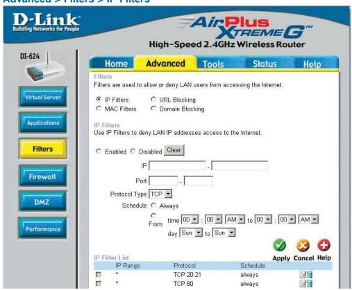
Filters are used to deny or allow LAN (Local Area Network) computers from accessing the Internet. The VDI-624 can be setup to deny internal computers by their IP or MAC addresses. The VDI-624 can also block users from accessing restricted web sites.
