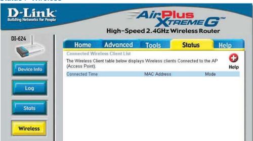
The wireless client table displays a list of current connected wireless clients. This table also displays the connection time and MAC address of the connected wireless client.
