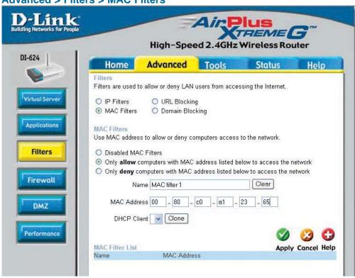
Use MAC (Media Access Control) Filters to allow or deny LAN (Local Area Network) computers by their MAC addresses from accessing the Network. You can either manually add a MAC address or select the MAC address from the list of clients that are currently connected to the Broadband Router.
