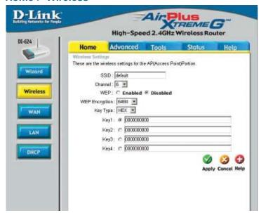
SSID- Service Set Identifier (SSID) is the name designated for a spe-
