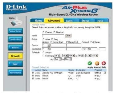
**Firewall Rules** is an advanced feature used to deny or allow traffic from passing through the VDI-624. It works in the same way as IP Filters with additional settings. You can create more detailed access rules for the VDI-624. When virtual services are created and enabled, it will also display in Firewall Rules. Firewall Rules contain all network firewall rules pertaining to IP (Internet Protocol).
