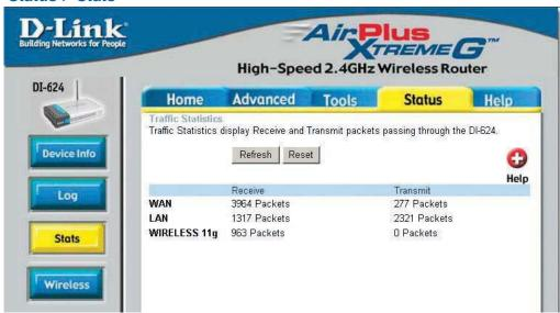
The screen above displays the Traffic Statistics. Here you can view the amount of packets that pass through the VDI-624 on both the WAN and the LAN ports. The traffic counter will reset if the device is rebooted.
