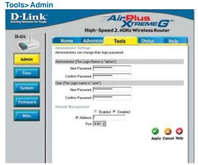
At this page, the VDI-624 administrator can change the system password. There are two accounts that can access the Broadband Router's Web-Management interface. They are admin and user. Admin has read/write access while user has read-only access. User can only view the settings but cannot make any changes.
