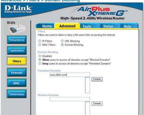
Domain Blocking is used to allow or deny LAN (Local Area Network) computers from accessing specific domains on the Internet. Domain blocking will deny all requests to a specific domain such as http and ftp. It can also allow computers to access specific sites and deny all other sites.
