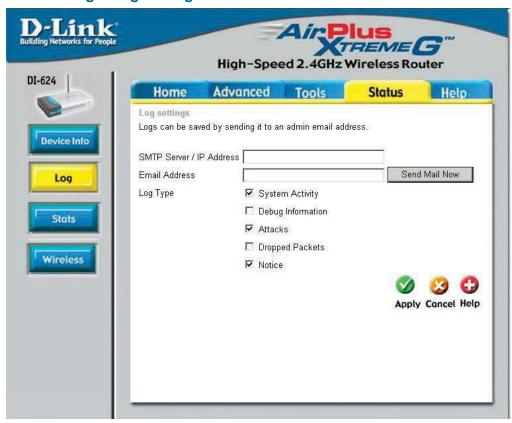
Not only does the Broadband Router display the logs of activities and events, it can be setup to send these logs to another location.
