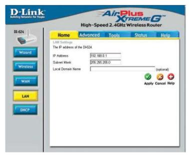
LAN is short for Local Area Network. This is considered your internal network. These are the IP settings of the LAN interface for the VDI-624. These settings may be referred to as Private settings. You may change the LAN IP address if needed. The LAN IP address is private to your internal network and cannot be seen on the Internet.
