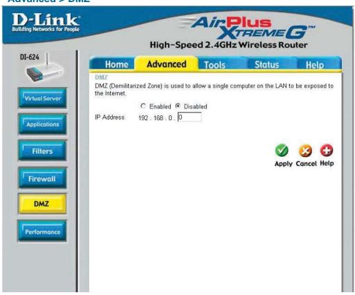
If you have a client PC that cannot run Internet applications properly from behind the VDI-624, then you can set the client up for unrestricted Internet access. It allows a computer to be exposed to the Internet. This feature is useful for gaming purposes. Enter the IP address of the internal computer that will be the DMZ host. Adding a client to the DMZ (Demilitarized Zone) may expose your local network to a variety of security risks, so only use this option as a last resort.
